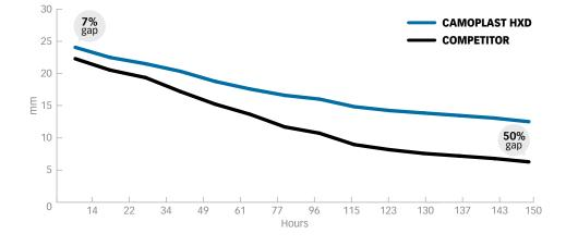
Camoplast tracks are designed with much thicker tread than most OEM tracks. Maintaining more rubber around the carcass offers more protection on carcass puncture and edge cutting. This all translates in longer service life and less downtime. The end result of this test is: **Camoplast HXD offers 30% more service life**.
