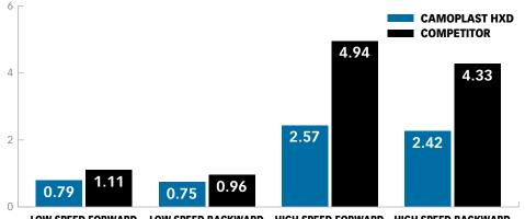
Throughout the entire test, the **vibration level was 42% lower with the Camoplast tracks** than the OEM quality track regardless the speed and the direction.
